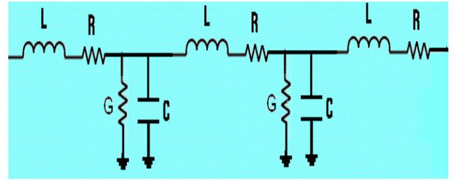
Figure 1: RLC model of an interconnect
